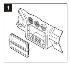
Disconnect the negative battery terminal to prevent an accidental short circuit. Unclip the radio trim bezel. Remove (4) 7mm hexhead screws securing the factory head unit and disconnect the wiring.
